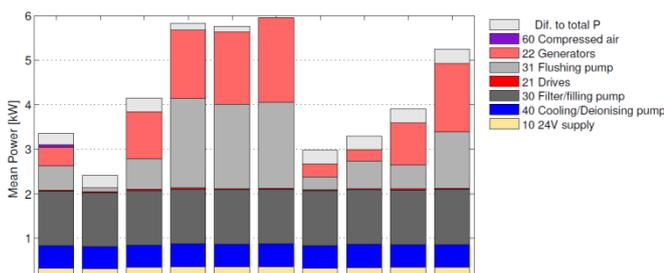
Fig. 2. Multichannel measurement on the CUT200 machine tool in different machine tool modes and machining processes.
