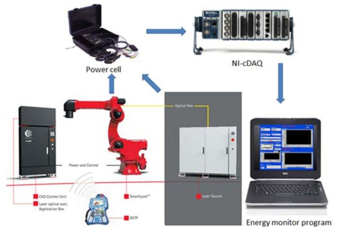
Figure 6. Measurement equipment of laser welding
